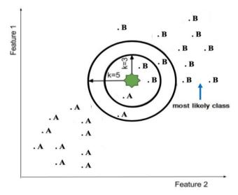
**Figure 4.** Example of kNN classifier for a two-class problem (i.e. dots annotated with A and B) for different values of K parameter (k=3, k=5). The green star represents a sample point for which the most likely class is needs to be determined
