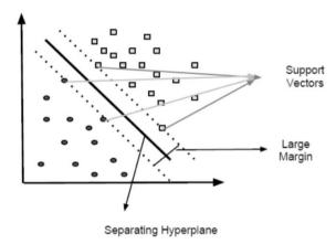
Figure 5. Illustration of a Support Vector Machine (SVM) [20]
